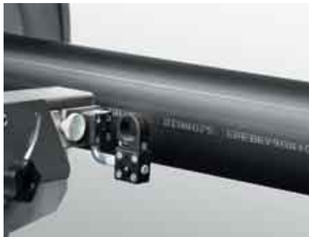
White ink coding on black tubing with 9232 E at Buxoplas Manufacturing.
