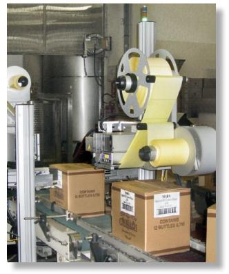
Depending on the type of production, 2000 Series systems allow two labels to be applied onto two adjacent sides of a box.
