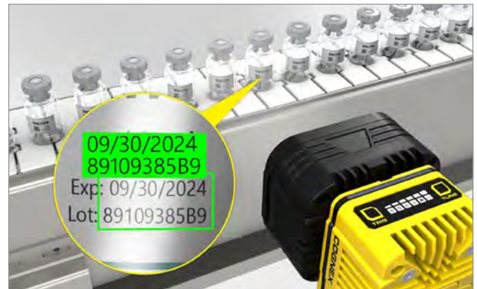
Pharmaceutical: Perform on-line verification at high speeds
