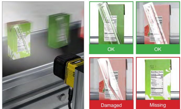
Food & beverage: Identify damaged or missing components
